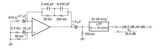
Figure 3 Noise Measurement Circuit (FLAT+JIS A)
