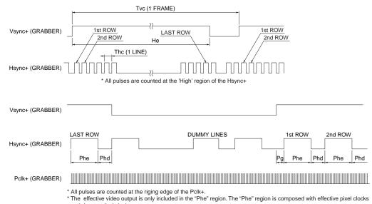
and dummy pixel clocks. \* Pclk always flows out regardless of the status for Vsync or Hsync.
