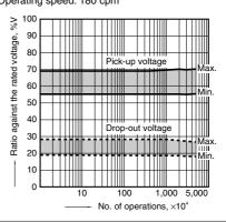
4. Electrical life (1 A 30 V DC resistive load) Tested sample: TXS2-4.5V. 6 pcs.
